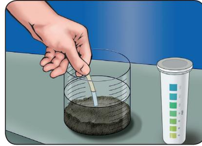
Use the manufacturer's instructions for the EM Quant QAC test sticks to analyze each slurry solution/extraction.
