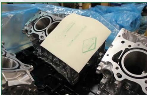
**VpCI®-130 Series** - Unique, flexible packaging materials that combine VpCI® protection, cushioning, and desiccant action, plus excellent antistatic capabilities all in one step! Cortec® VpCI®-130 Series Foams provide effective corrosion protection. Patented.
